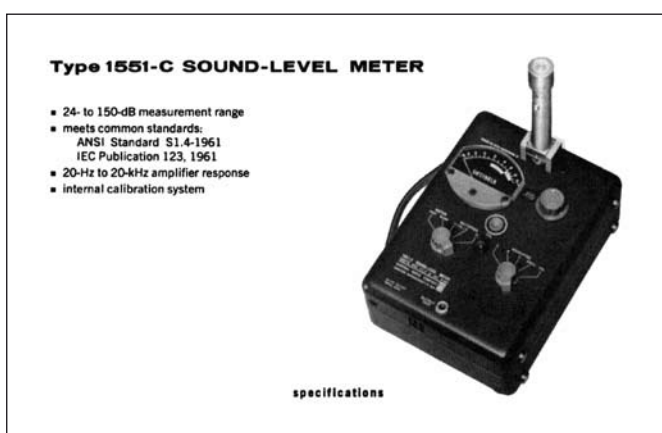
Fig 2. An early sound level meter used by the author [GenRad 1963]
